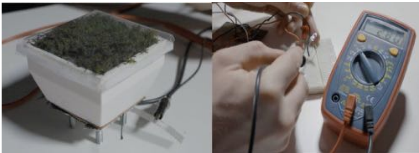
Figure 14: An early moss-based microbial fuel cell prototype for Le Centre Pompidou (2021). Photo by Guillaume Pascale.
