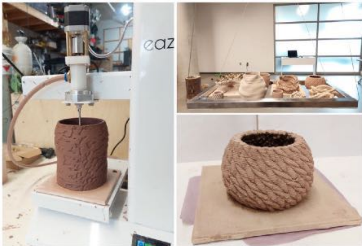
Figure 29: Ceramic 3D printing research with an Eazao Zero extrusion printer (left), 3D printed ceramic planters developed while conducting research (right). Photos by the author (2023).
