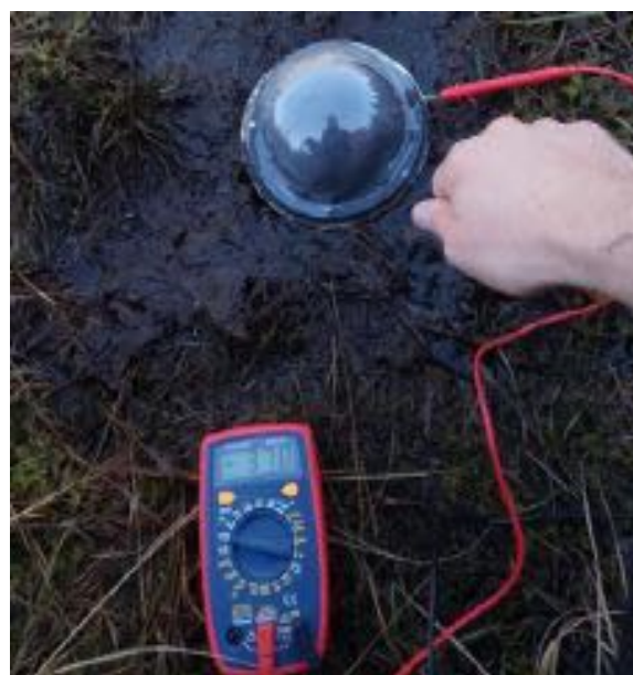
Figure 11: An early anaerobic MFC prototype measuring the real-time energy output of its component’s energy harvesting processes. Photo by the author (2021).
