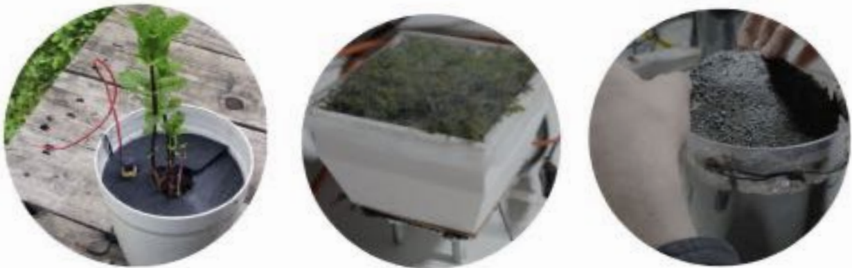
Figure 8: Varying types of MFCs: a P-MFC (left), a Bryo-MFC (center), and an Anaerobic MFC (right). Photos by Johann Duraffourg (left, 2017) and Guillaume Pascale (center & right, 2022).
