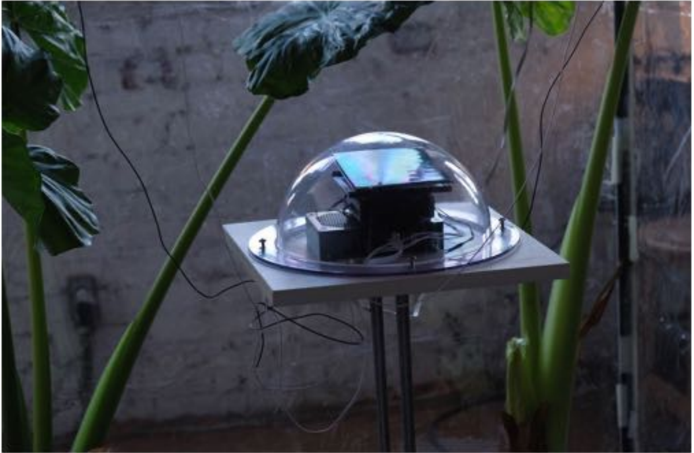
Figure 41: The installation's solar server setup – the modular 3D cases, plinth, and acrylic dome - used within the installation exhibition. Photo by the author (2024).
