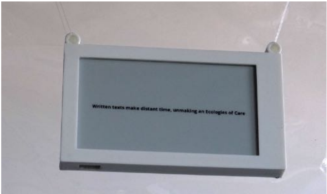
Figure 33: An E-Ink module within the installation, enclosed within a custom 3D printed mounting case for the installation. Photo and design by the author (2024).
